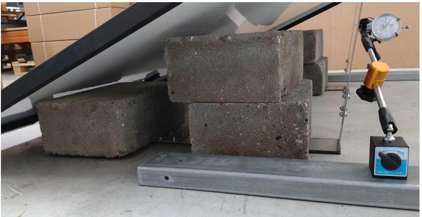
Figure 1. Configuration of the PV panel support strength test bench
