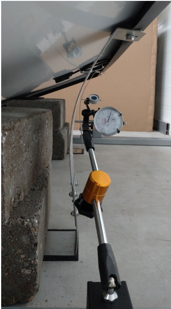
Figure 4. Deformation of the support leg at a maximum load of 448 kg (picture left) and after load removal of 0 kg (picture on the right)
